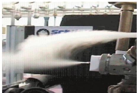
Image 2: Dust particles are kept away from the new air cap, instead of adhering to it
